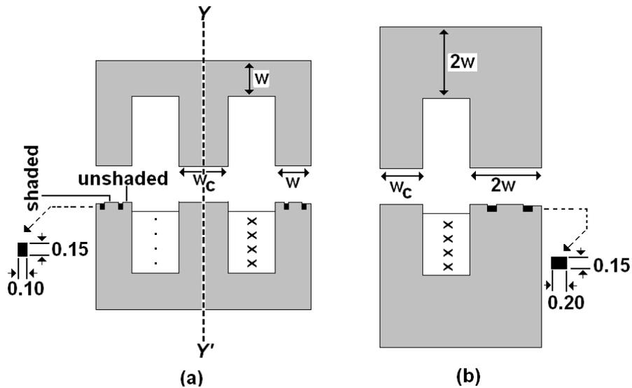
Figure 3. (a) Cross-sectional view of the contactor; (b) Simplified magnetic structure.
