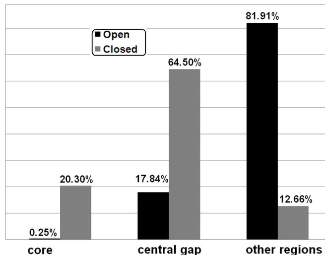
Figure 13. Per cent values of stored energy in different regions of the contactor's numerical model.
