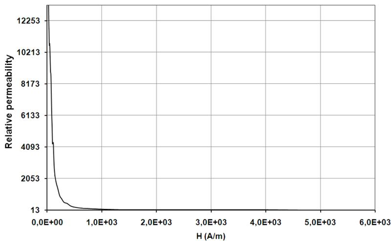
Figure 7. Variation of relative permeability as a function of the H-field for the “Carpenter Silicon Core Iron A, 1066C Anneal” composite.
