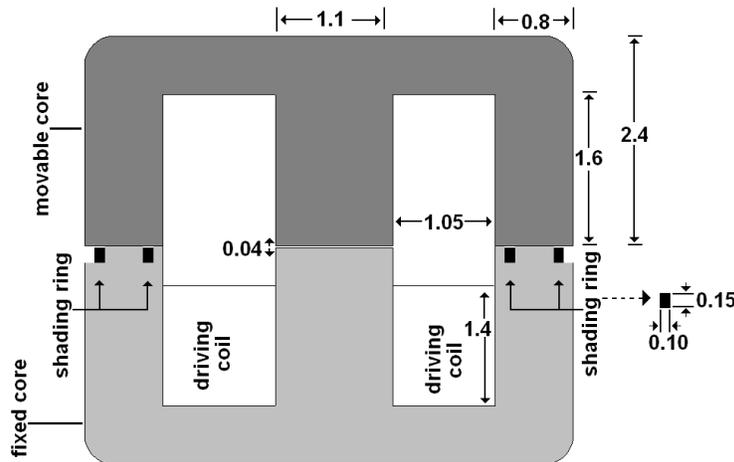
Figure 2. Sketch of the contactor’s electromagnet, dimensions in centimeter. Not to scale.
