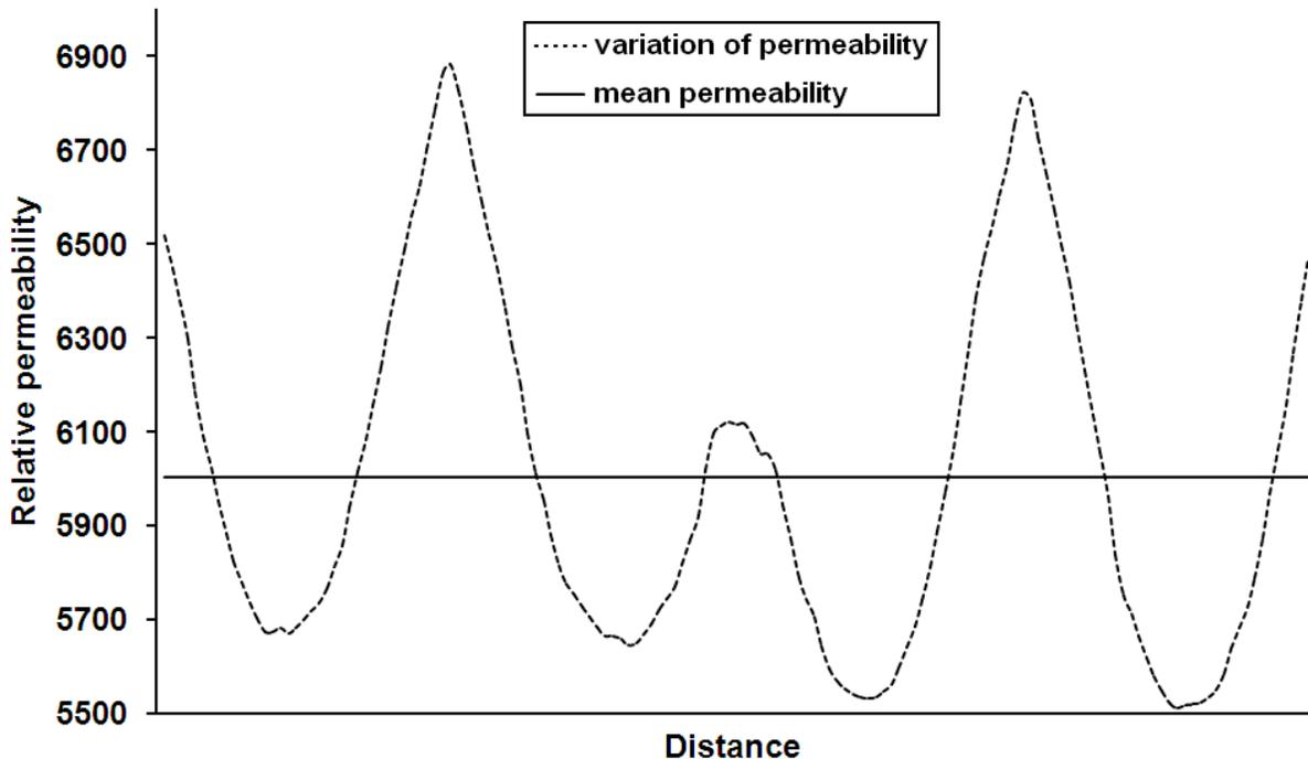
Figure 8. Averaged value and variation of the relative permeability along the outer limbs of the simplified magnetic structure.
