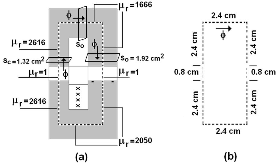
Figure 9: (a) Cross-sectional view of the simplified magnetic structure, and computed relative permeabilities;(b) Mean flux path lengths;
