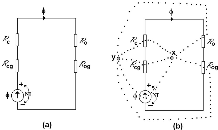
Figure 10. (a) Reluctance model for the contactor's open configuration; (b) Creation of the magnetic-electrical dual circuit.
