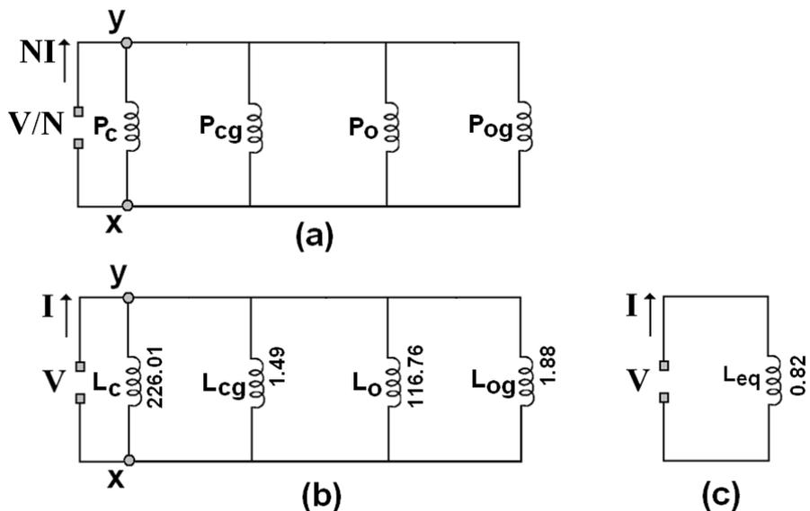
Figure 11. (a) Intermediate electrical dual circuit or permeance model; (b) Final electrical dual circuit; values of inductors in henry; (c) Final electrical dual circuit with the equivalent inductor.
