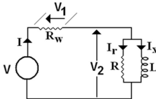
Figure 4: Conventional equivalent electric circuit of the contactor.
