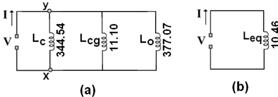
Figure 12. (a) Electrical dual circuit for the contactor's closed core configuration; (b) Dual circuit with the equivalent inductor.
