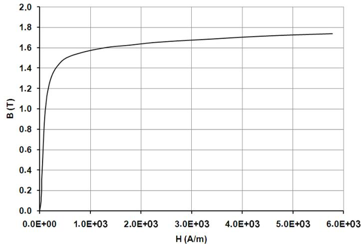
Figure 6. B-H curve for the composite material commercially known as “Carpenter Silicon Core Iron A, 1066C Anneal”.
