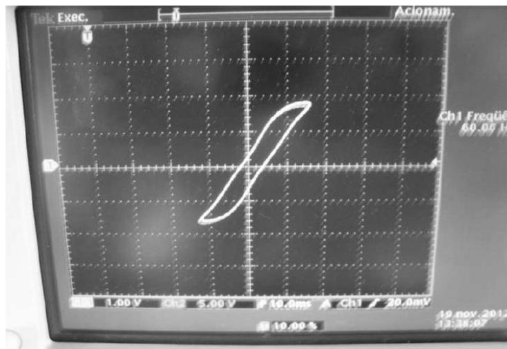
Figure 5. Hysteresis loop of the contactor’s bulk lamination for an applied overvoltage of 13.6%.
