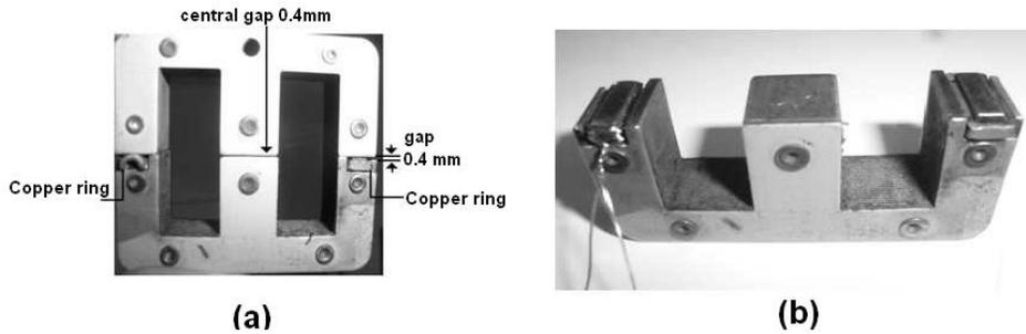
Figure 1. (a) The magnetic core at closed position; (b) Details of the fixed-core laminations.
