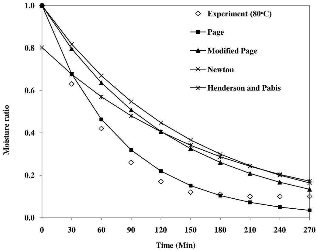
Figure 7. Models prediction with the experimental data at 80°C for 3 mm thickness
