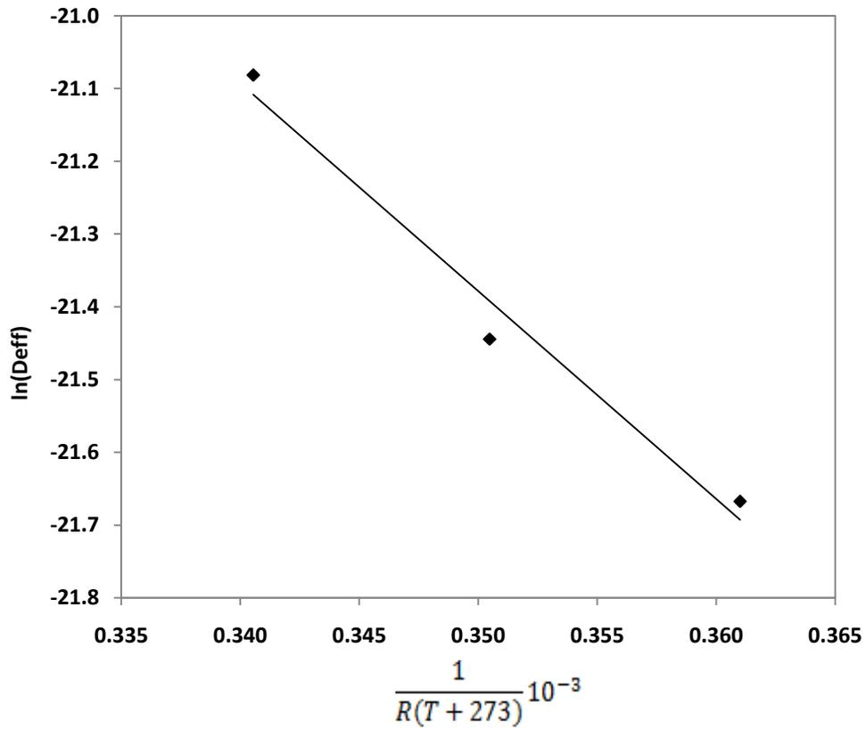
Figure 9. Estimation of Activation Energy
