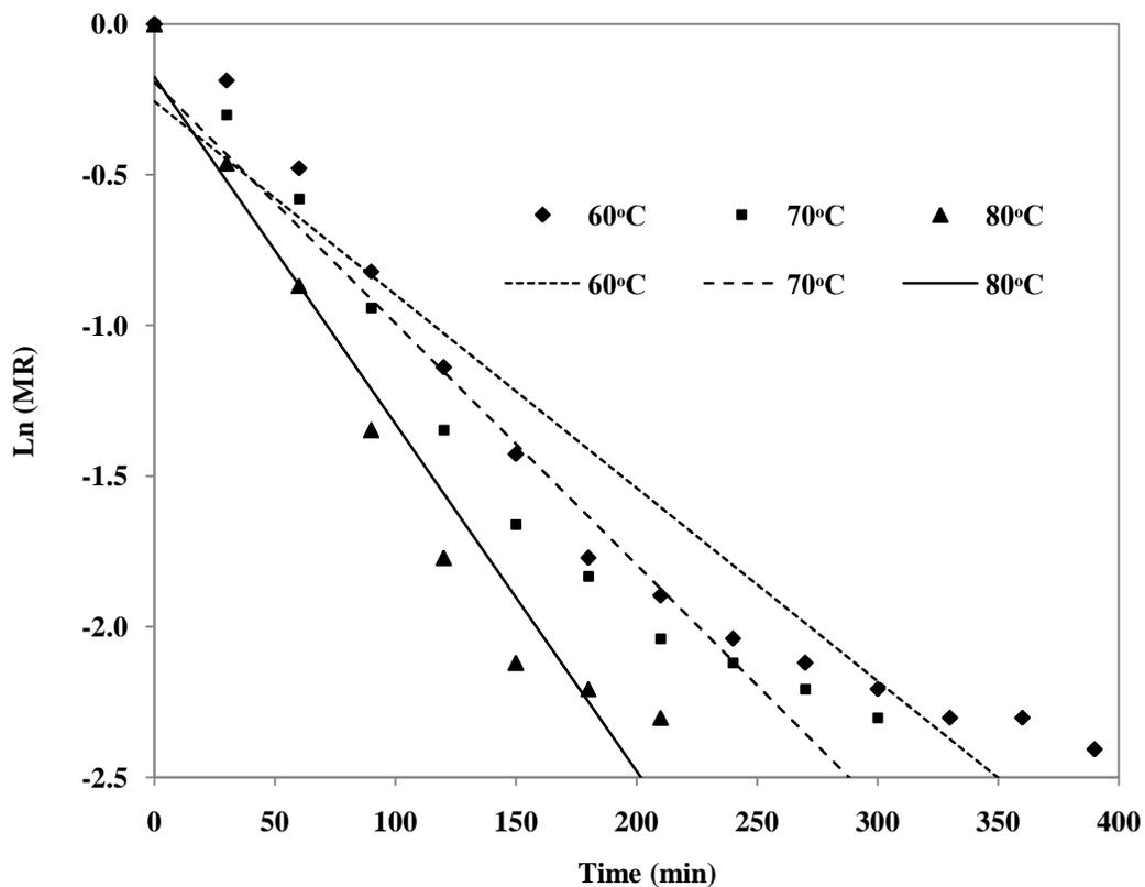
Figure 8. Estimation of Moisture Diffusivity Coefficient
