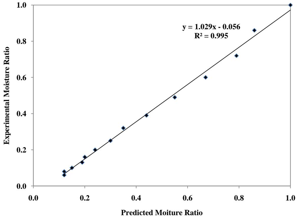
Figure 5: Page model fitting for 80°C, 3 mm slice thickness
