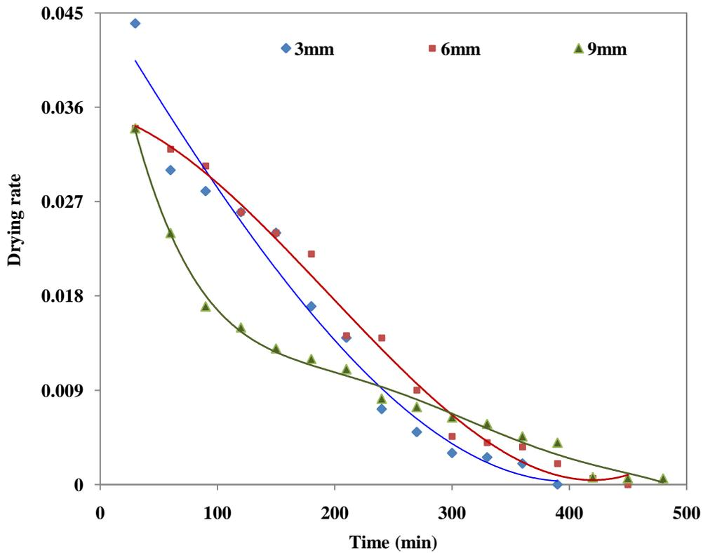
Figure 4: Drying rate curves for mango at different slice thicknesses
