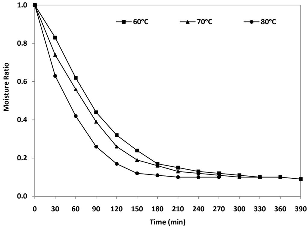
Figure 1: Effect of drying air temperature for 3 mm thick slices
