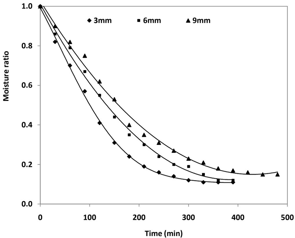
Figure 2: Effect of slice thickness on drying at 70°C drying temperature
