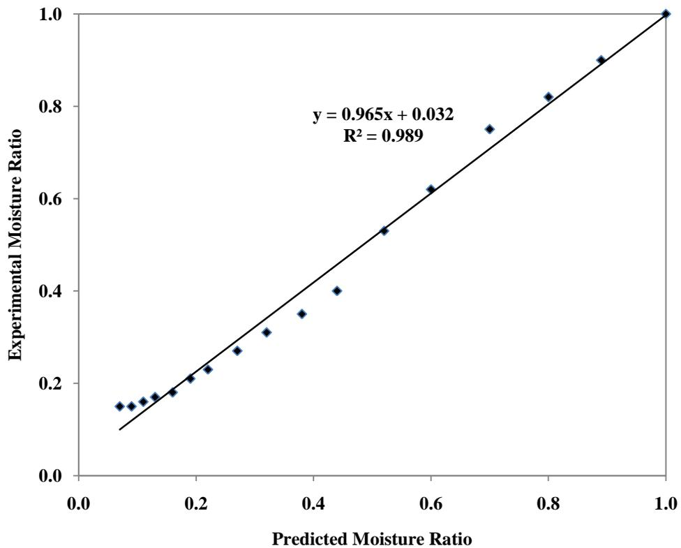
Figure 6: Page Model fitting for 70°C, 9 mm slice thickness
