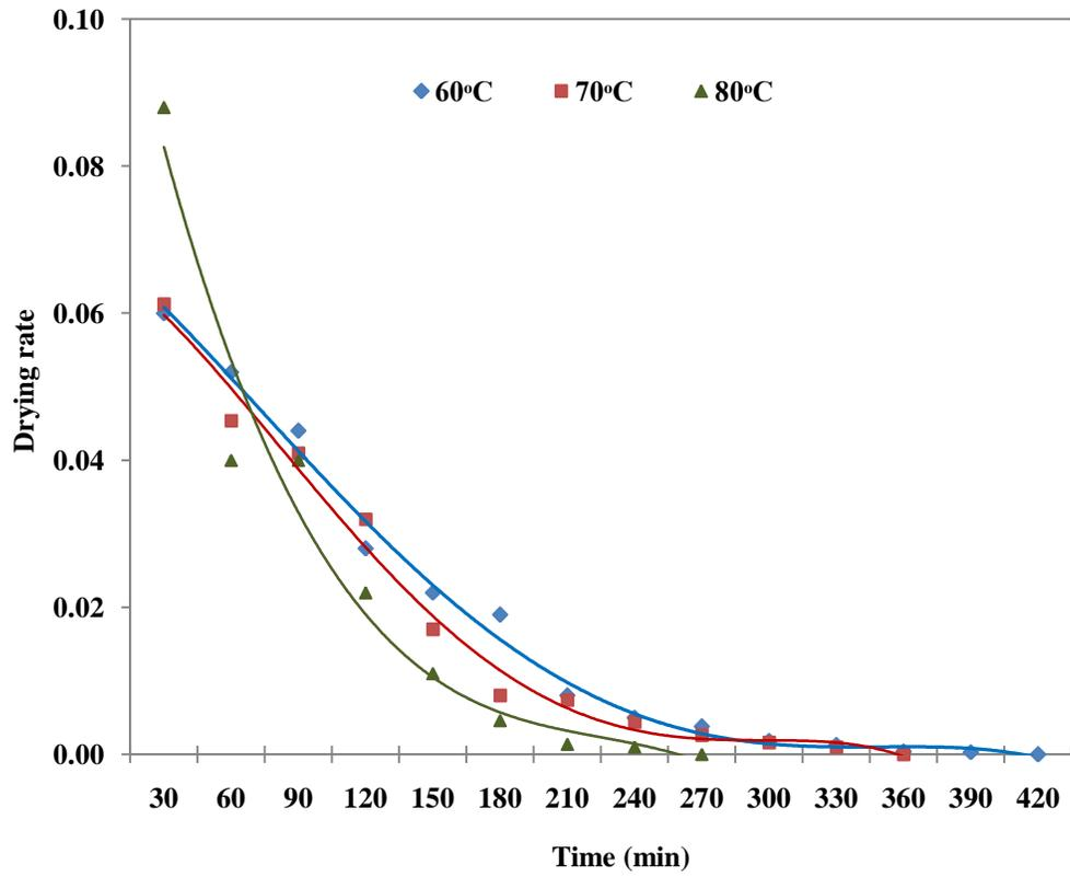
Figure 3: Drying rate for mango slices at different temperature setting.
