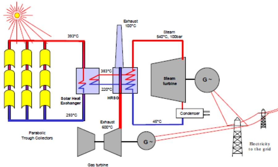
*Figure 4: Scheme Parabolic Trough Solar Power Plant at Hassi R'mal [23]*
