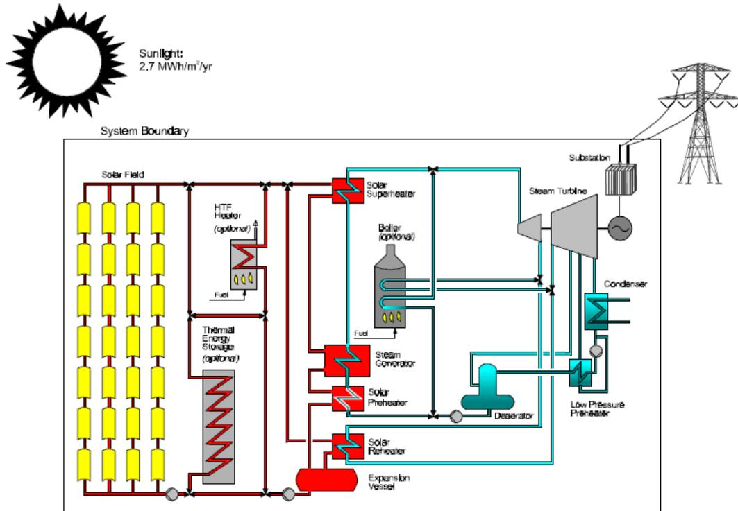
**Figure 3:** Scheme of Solar energy generating system in California [16].
