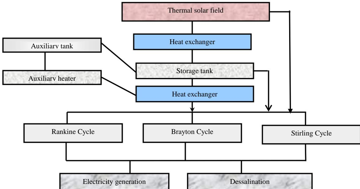
**Figure 2:** solar thermal technology
