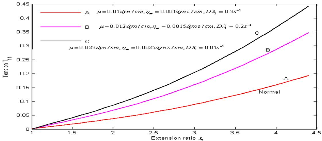
**Fig. 3.8: Stress versus strain and rate of strain curves in uniaxial tension. The different curve shows various values of the parameters and strain rate using equation (49) [38]**
