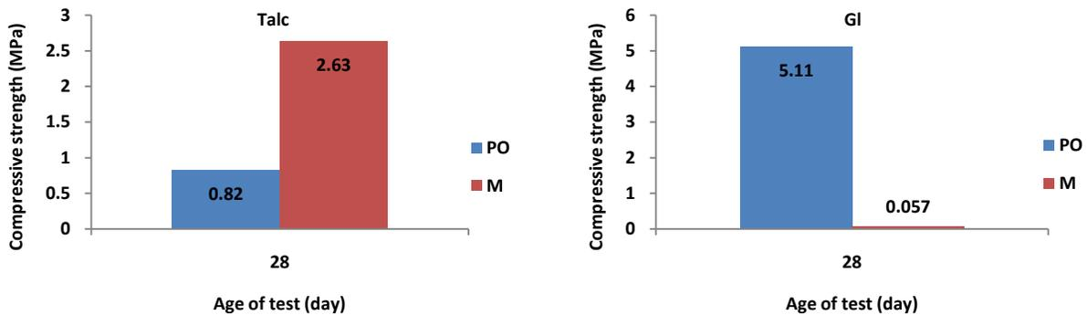
Figure 12. Comparison between compressive strengths of concrete based on different types of cement and superplasticizer, Left: Talc, Right: Glenium
