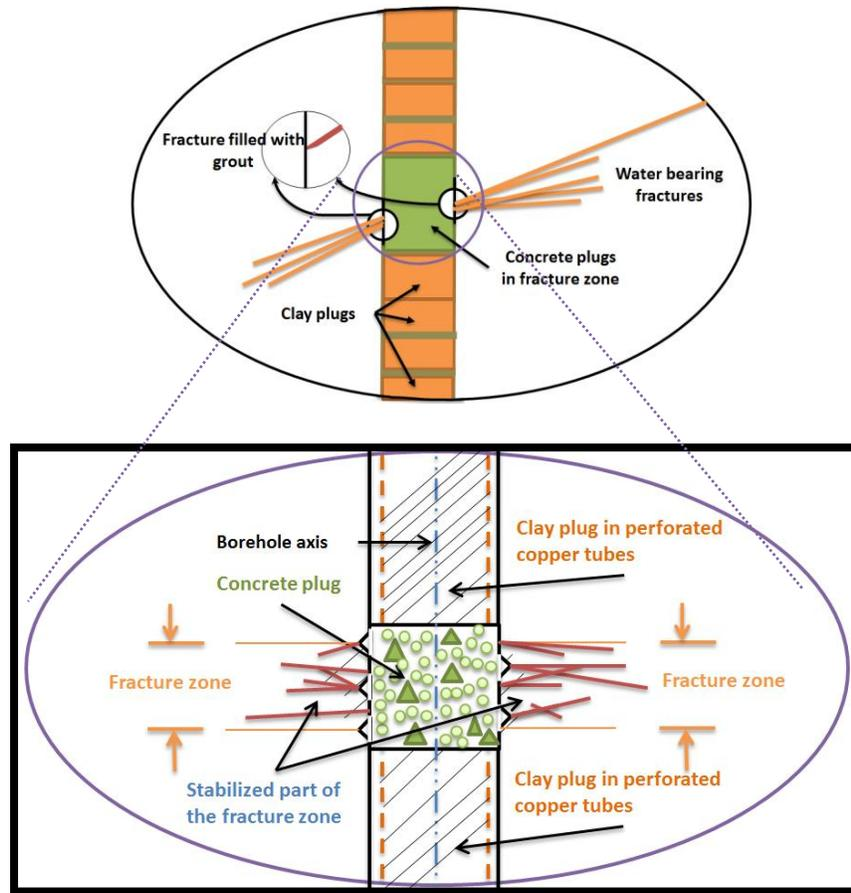
Figure 1. Upper: Principle of borehole sealing. Lower: Detail of concrete cast where the borehole intersects a fracture zone.
