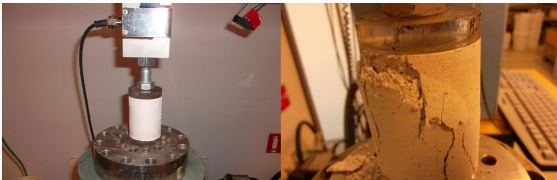
Figure 8. Uniaxial compression test
