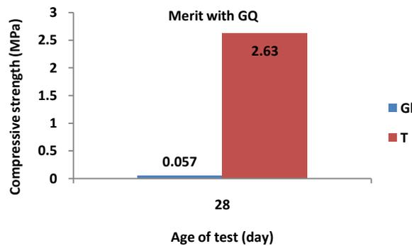
Figure 11. Comparison between compressive strengths of concrete with Merit cement and different superplasticizers
