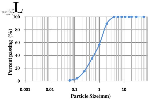
Figure 3. Grain size analysis of crushed quartzite
