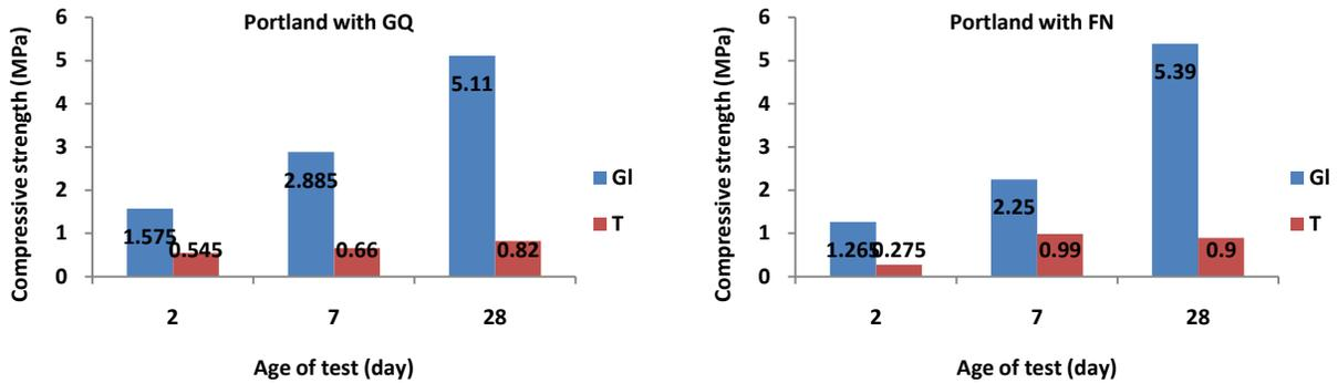
Figure 10. Compressive strengths of Portland concrete with different superplasticizers and fine aggregate, Left: Ground quartzite, Right: FN
