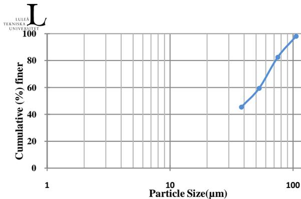
Figure 5. Grain size analysis of ground crushed quartzite
