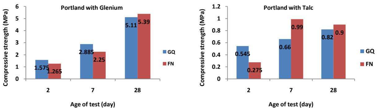
Figure 9. Compressive strengths of concretes based on Portland cement and different fine aggregate types with superplasticizer, Left: Glenium, Right: Talc
