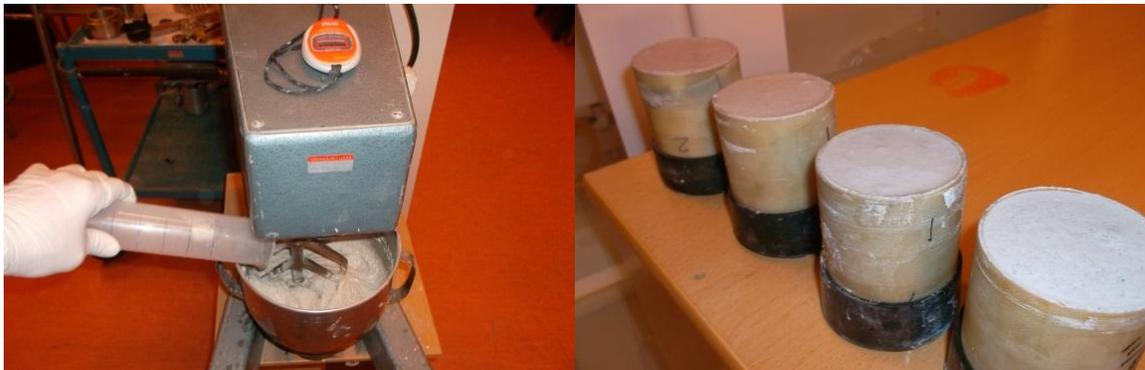
Figure 7. Left: Concrete mixture preparation demonstrating fluidity, Right: Molded samples
