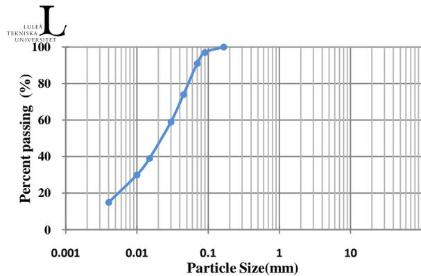
Figure 4. Grain size analysis of fine aggregate component
