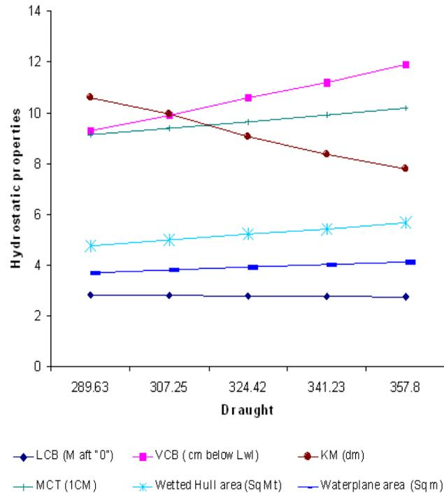
Fig. 5: Hydrostatics curves
