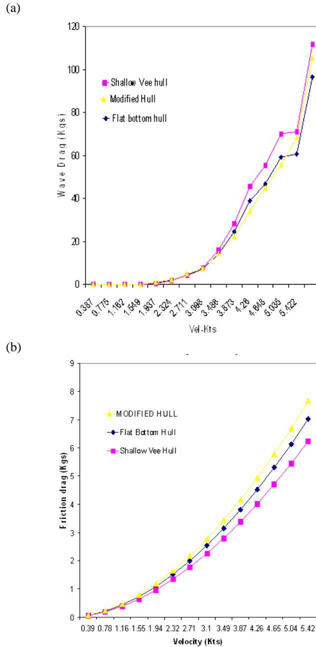
Fig. 7: The wave drag and friction drag as a function of velocity (a) The wave drag vs. velocity (b) . Friction drag vs. velocity
