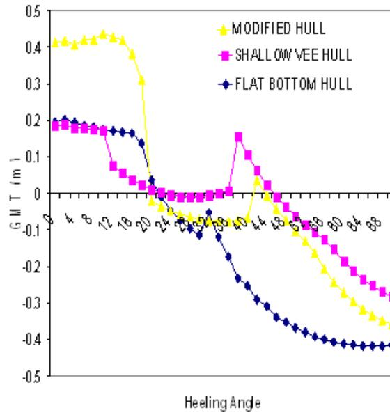
Fig. 10: The value of transverse of GMT verses heeling angles
