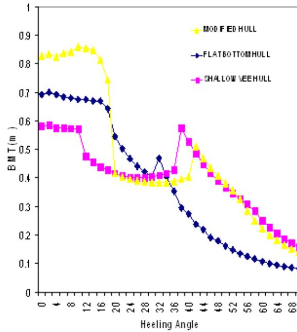
Fig. 9: The value of transverses of BM versus heeling angles
