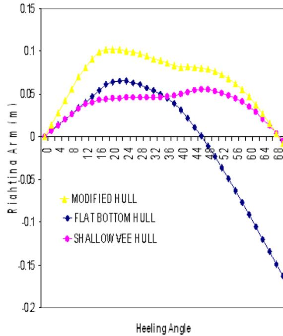
Fig. 8: The value righting arm Vs. heeling angle curves
