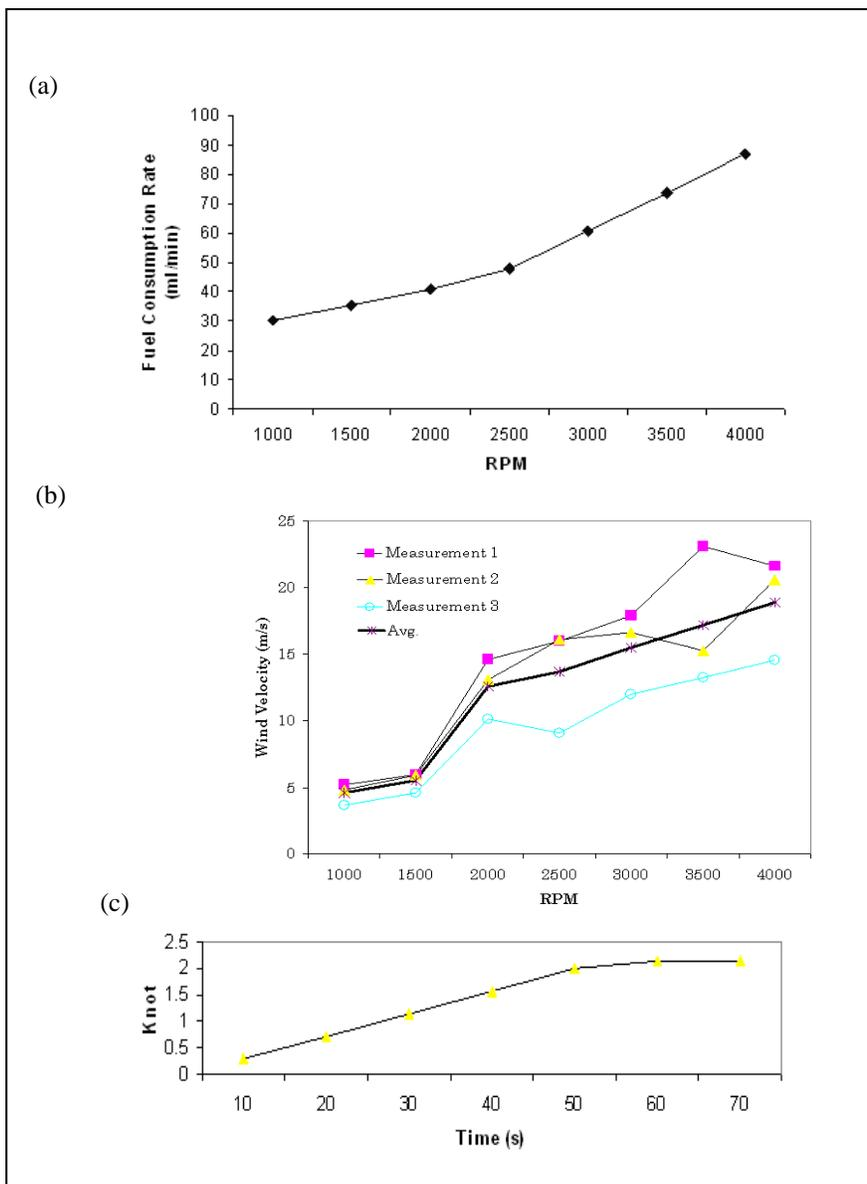
**Fig. 4:** Some typical airboat performance tests (a) typical fuel consumption rate vs. rpm; (b) Wind speed vs. rpm; and (c) airboat speed vs. time.
