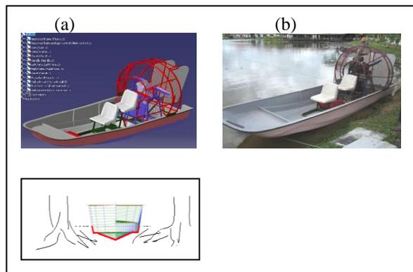
**Fig. 3:** The airboat design investigation. (a) Water level is analyzed by the CATIA design software program (left picture); (b) rail is installed on the airboat for ease of frame adjustment (right picture); (c) a typical schematic sketch of a narrow mangrove habitat versus the Vee hull shape boat outline
