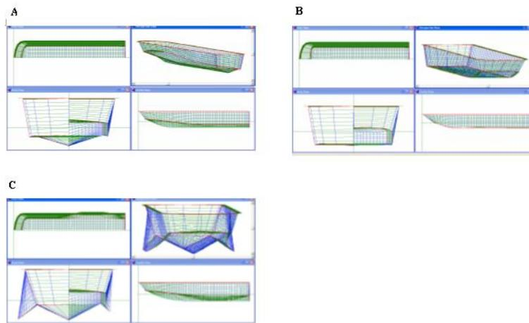
Fig. 6: Various hull types drawn with B-splines drawing. (a) The Shallow-Vee; (b) Flat Bottom; and (c) Modified hull.
