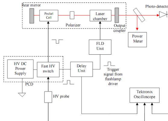
Figure 4: Experimental setup of high voltage power supply for electro-optics applications.
