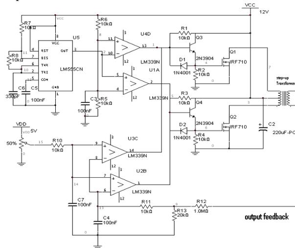
Figure 2: The schematic diagram MOSFET driver circuit
