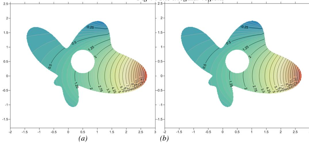
Fig 5. The field potential solutions: (a) exact results and (b) proposed method
