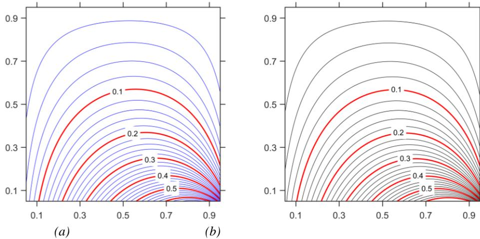
Fig 2. The field potential solutions: (a) exact results and (b) proposed method
