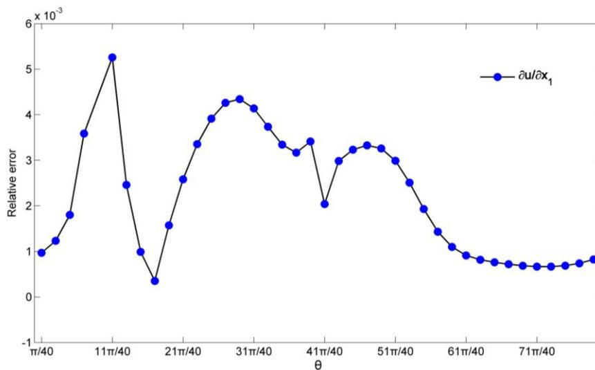
Fig 6. The relative errors for the flux  $\partial u/\partial x_1$  on the boundary  $\Gamma_2$
