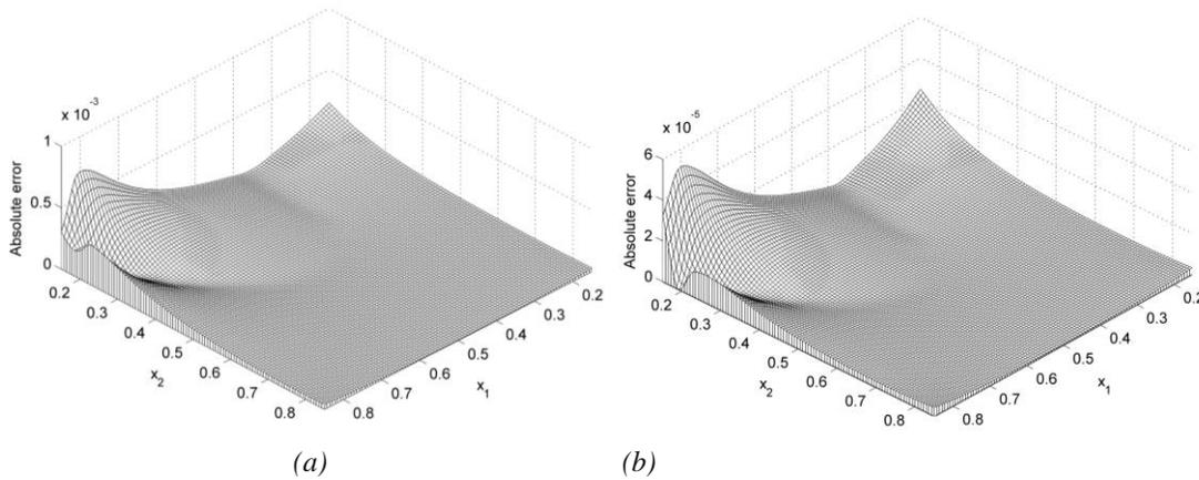
Fig 3. Absolute error surfaces for field potential solutions, where the number of boundary element is 40 for (a) and 80 for (b), respectively.
