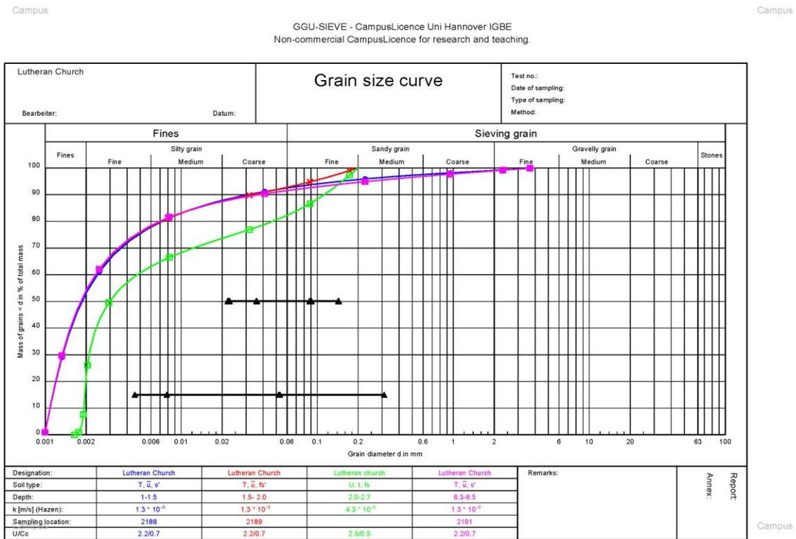
Figure 4: Grading curves for soils samples recovered at Lutheran Church site
